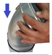
3. Encase the fitting inside the duct and press till full interlocking. For an easy mounting, we recommend the use of Vaseline or industrial grease.
