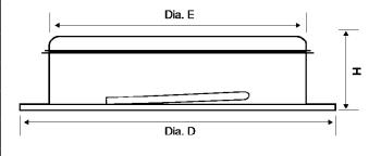
Tolerance : +/- 3 mm except Dia E: Tolerance: +/- 1 mm
