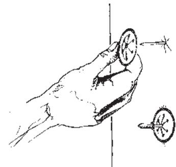
Insulation can be impaled immediately and firmly locked with locking washers, but maximum strength of adherence is achieved afetr 24 hours. If necessary, cover the pin with protective cap.
