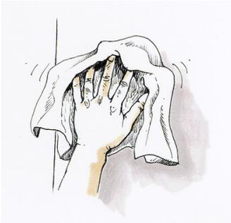
Apply at temperature range +15°C to +25°C (+60°F to +80°F). Surfaces should be clean and dry, free of dust, grease, oil and any other loose matter. Do not use dissolvent products. Not for use in application likely to make contact with chlorinated, cetonic or esther solvents.
