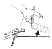
Fix earth clamp of the welder to the sheet metal.
