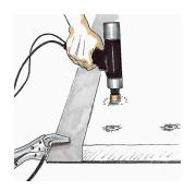
Press the fastener through the insulation until the tip of the shank meets the sheet metal and press the trigger
