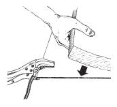
Fix earth clamp of the welder to the sheet metal.
