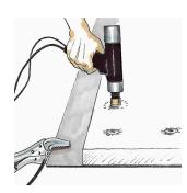
Press the pin through the insulation until the tip of the shank meets the sheet metal and press the trigger
