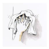
Apply at temperature range +15°C to +25°C (+60°F to +77°F). Surfaces should be clean and dry, free of dust, grease, oil and any other loose matter. Do not use degreasing products. Not for use in application likely to make contact with chlorinated, cetonic or esther solvents.
