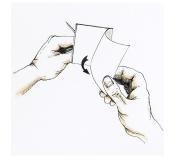
Remove the protective release paper taking care not to touch the adhesive
