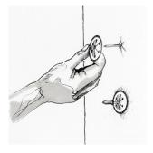
If necessary, cover the pin with protective cap.
