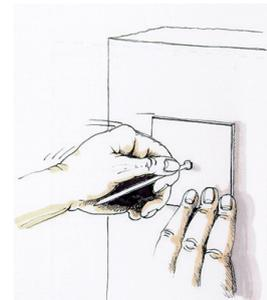
Place the hanger in the required position and press the base against the surface to be insulated
