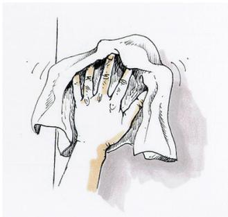
Apply at temperature range +15°C to +25°C (+60°F to +80°F). Surfaces should be clean and dry, free of dust, grease, oil and any other loose matter. Do not use degreasing products. Not for use in application likely to make contact with chlorinated, cetonic or esther solvents.
