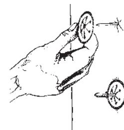
Insulation can be impaled immediately and firmly locked with locking washers, but maximum strength of adherence is achieved after 24 hours. If necessary, cover the pin with protective cap.
