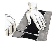
Lift the seam outwards at right angle
