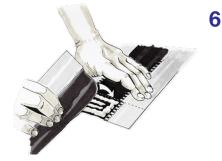
Coat the cloth with the appropriate adhesive or use our self-adhesive pads (if appropriate). Join both sides and press together firmly
