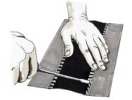
Lift the seam outwards at right angle
