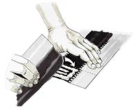
Coat the cloth with the appropriate adhesive or use our self-adhesive pads (if appropriate). Join both sides and press together firmly
