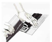
Coat the cloth with the appropriate adhesive. Join both sides and press together firmly
