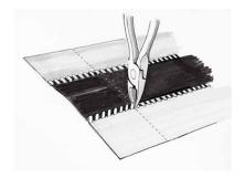
Make a cut at the edge of the lifted seam
