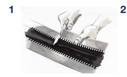
At a notch, cut a length equivalent to the perimeter required plus an overlap of 2" (5 cm) for joining
