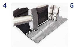
Bend down the seam whilst ensuring that the cloth remains fastened
