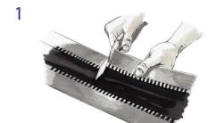
At a notch, cut a length equivalent to the perimeter required plus an overlap of 5 to 6 cm (2") for joining
