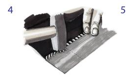
Bend down the seam whilst ensuring that the cloth remains fastened
