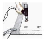
Press the pin through the insulation until the point meets the sheet metal and press the trigger
