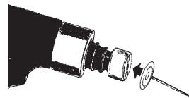
Place the weldfastener CDF on the magnetic head of the gun.
