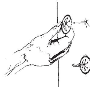
Insulation can be impaled immediately and firmly locked with locking washers, but maximum strength of adherence is achieved after 24 hours. If necessary, cover the pin with protective cap.
