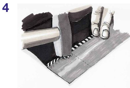
Bend down the seam whilst ensuring that the cloth remains fastened
